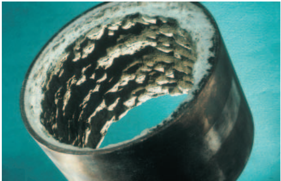
Figure 1.4 Hard water causes mineral deposits called scale to form on the inside of pipes. The scale clogs up the pipes.
