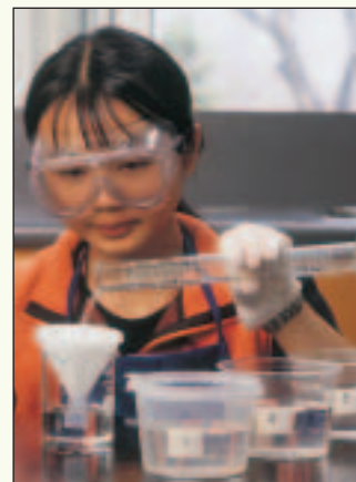
Figure 1.6 Step 3. Pour 100 mL of one water sample through the filter.
