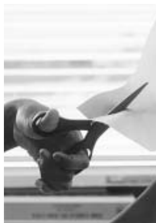
Figure 1.18 To cut, you move the scissors' handles together. The scissors' blades cut the paper more quickly than you move the handles together. And they cut farther than the distance the handles move. Try it and see!
