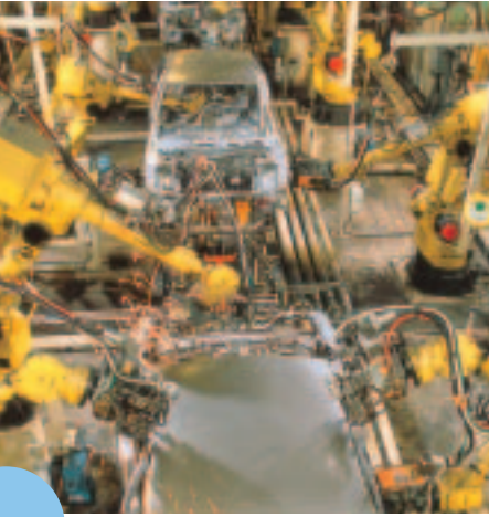
Figure 3.17 Assembly-line robots weld car bodies together in an automobile factory.
