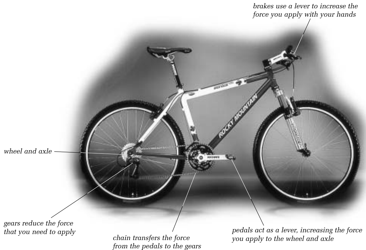
Figure 1.22 A bicycle is a complex machine made up of simple machines that work together. The whole bicycle is a system, made up of many subsystems.
