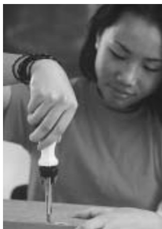
Figure 1.17 A small force on the handle of the screwdriver becomes a large force in the shaft. This large force can then be used to undo screws that would be impossible to remove with your fingers alone.
