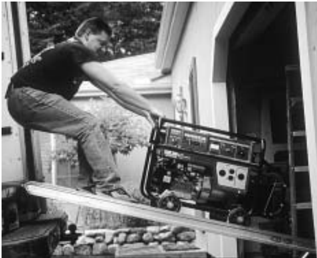
Figure 1.7 An inclined plane or ramp can help move large, heavy objects that are too heavy to lift straight up.
