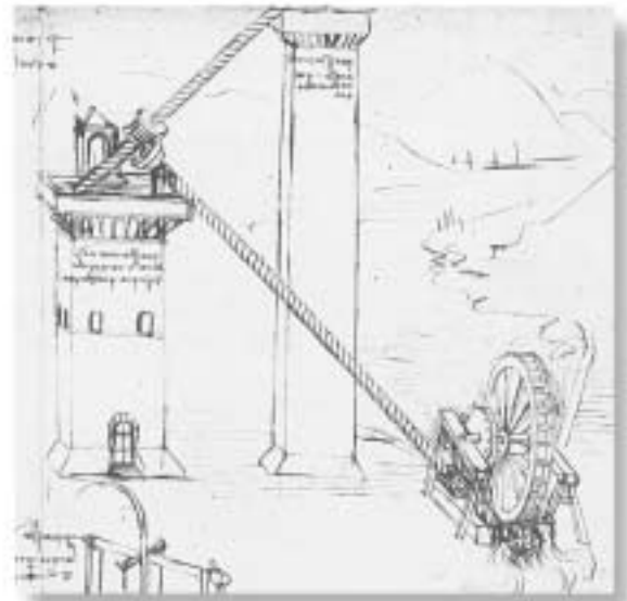
Figure 1.3 Leonardo da Vinci's design for using two Archimedes screws to raise water up into a water tower.
