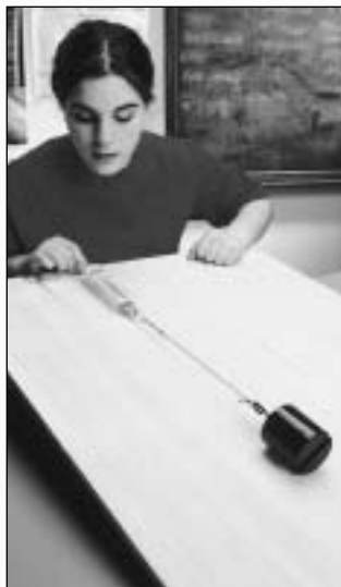
Figure 1.13 Step 4. Pull the mass steadily up the ramp.
