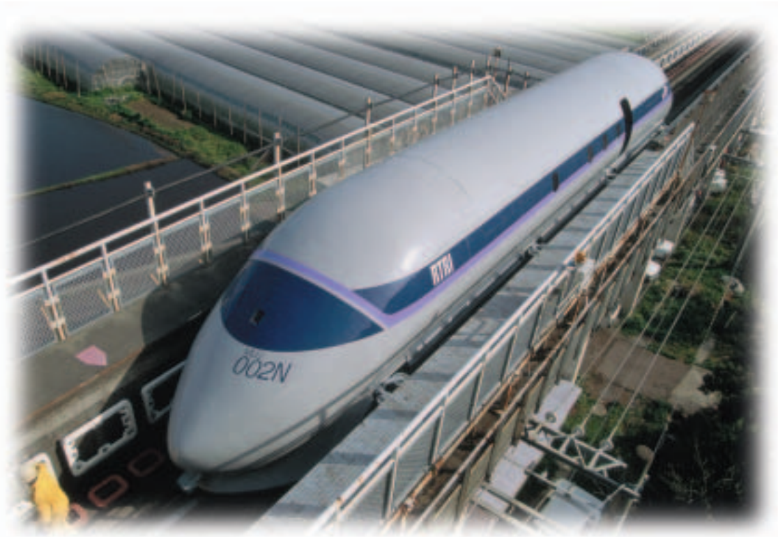
Figure 3.15 Because they float on magnets, MAGLEV trains experience very little friction. This enables them to use more of their energy for increasing speed rather than opposing friction.
