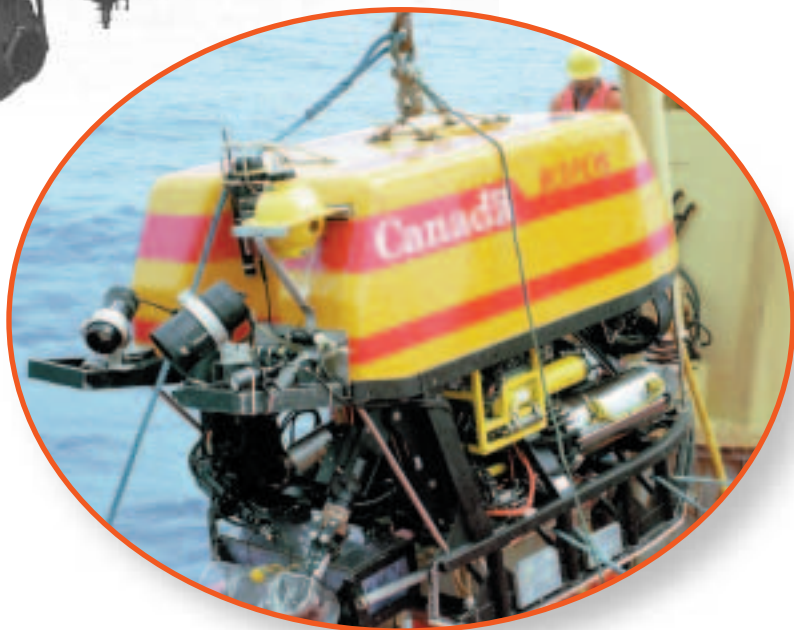
Figure 4.12 This submersible robot ROPOS is equipped with two robotic arms and can dive to 5000 m.
