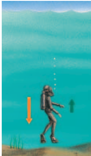
Figure 3.10a) The diver is able to move downward because of a combination of forces. The force of gravity acting on her, along with the force of her leg movement, is greater than the buoyant force of the water.
