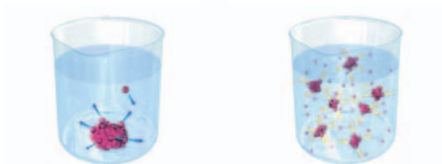
Figure 2.13b) Size of Pieces. Small pieces of solute dissolve more quickly than large pieces. All the smaller pieces together have more surface area among them for the solvent particles to bump into. Think of cooking a potato in water. If you put the whole potato in, it takes a long time to cook. If you cut the potato up into smaller pieces, the cooking time becomes much shorter.
