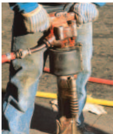
Figure 1.11 This jackhammer is pneumatic. Systems that use compressed air are called pneumatic systems . Hydraulic systems use liquids to lift or move things. You will learn more about pneumatic and hydraulic systems when you learn about the compression of fluids in sections 3.0 and 4.0.
