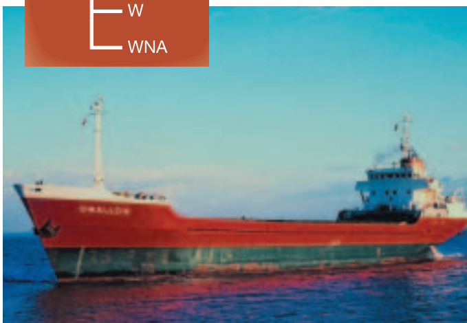
Figure 3.11 The Plimsoll line indicates how heavily loaded a ship can be in different densities of water.
