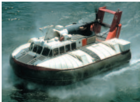
Figure 1.12 The hovercraft operates by directing air downward so it floats on a fluid cushion over the waves.
