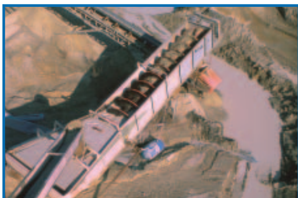
Figure 4.5 The Archimedes screw is a pump supposedly invented by Archimedes to remove water from the hold of a ship. Here it is used as a sand washer on a construction site.
