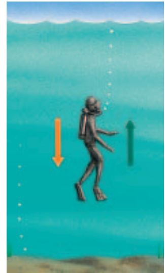
Figure 3.10c) The diver can float suspended in the water where the force of gravity equals the buoyant force. This situation is called neutral buoyancy .
